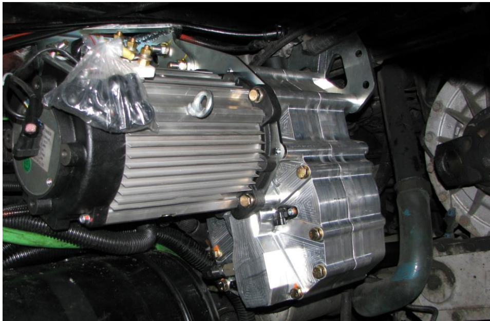
Gearbox and System Starter-Generator (rear view - main driveshaft removed )
